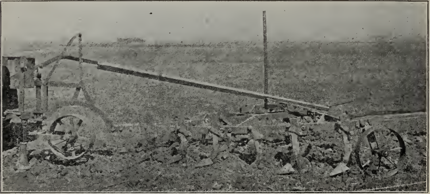
Fig. 10.—The Alameda Sugar Company at Alvarado, California, use this weeder, drawn by 80 h.p. Holt tractor, in preparation of morning glory infested beet land. It runs 10 to 12 inches deep.
